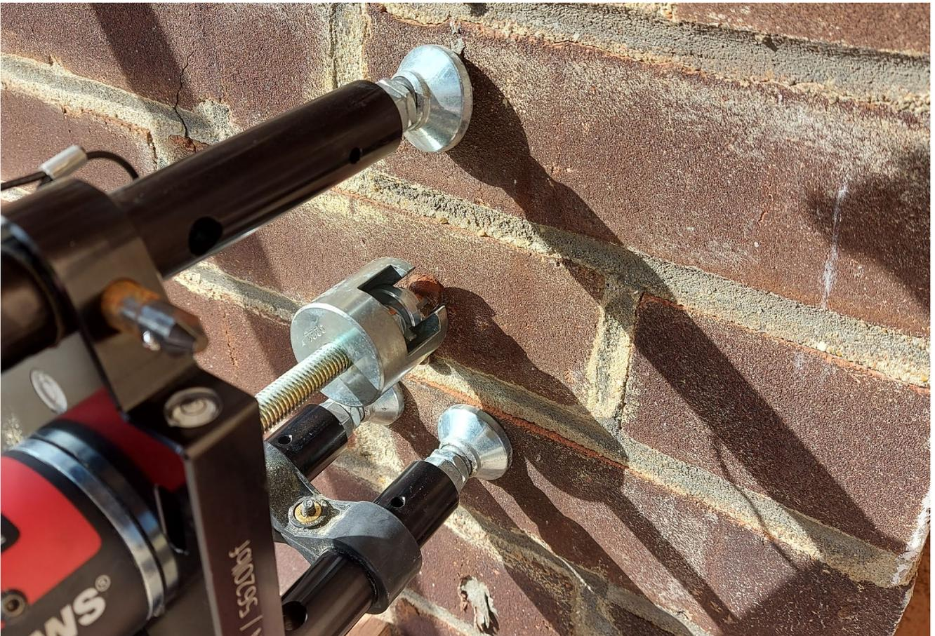
The bricks were drilled with a SDS-P-8.0\*210-P drill bit, with hammer drilling enabled. I did try without the hammer setting enabled but the brick is too dense for this.
